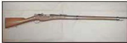
*Note in the picture above and also the carbines below that the magazine on the three round Berthier does not extend below the woodwork.*
