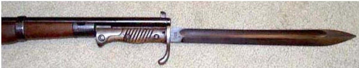
*Production of the Destroyer continued up until the early 1970's. The 9mmLargo cartridge was first loaded in Spain about 1907 and used in their Bergmann pistols hence it's use in the destroyer carbine. The Destroyer has a six round detachable magazine.*
