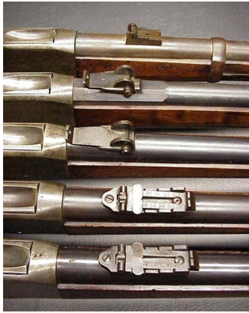
Peabody Rifle Rear Sights - Military Models, Top to Bottom: M1866 Canadian, M1867 Swiss (but with later Swiss-made and installed replacement barrel. Note that it has an octagonal knoxform. The original Swiss model Peabody has a round barrel; same sights), M1868 Roumanian (similar to the Swiss, leaf extends to the receiver), M1868 Spanish and M1870 Spanish (the Spanish sights are identical, but the calibre of the rifles (.50 and .43) are quite different. Also, the breech blocks are very different, see below).
