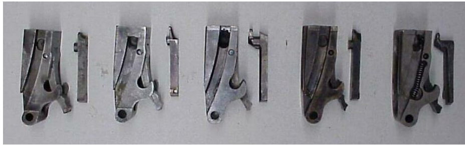
Peabody Rifle - Military Models - Breech Blocks Interior Construction, Left to Right: M1866 Canadian, M1867 Swiss, M1868 Roumanian, M1868 Spanish(?) and M1870 Spanish (the Spanish model is the significantly different one, with a spring loaded firing pin retraction system. Though difficult to see, the firing pin is also noticeably thinner at the hammer end than the other models. (See close-ups below)
