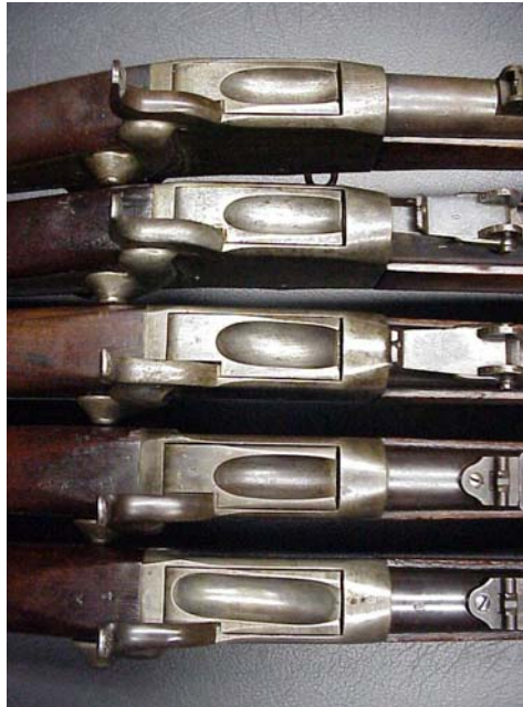
Peabody Rifle Top of Breech Blocks - Military Models, Top to Bottom: M1866 Canadian, M1867 Swiss, M1868 Roumanian, M1868 Spanish(?) and M1870 Spanish (the M1870 Spanish model is the significantly different one, with much longer and deeper breech block cartridge loading cut-out and thinner hammer. The others differ internally (see below), but are identical externally).
